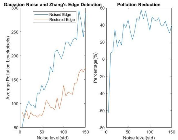
**FIGURE 6:** COMPARISON OF NOISE POLLUTION IN NOISED AND RESTORED EDGES FOR ZHANG EDGE DETECTION ALGORITHM [14]
