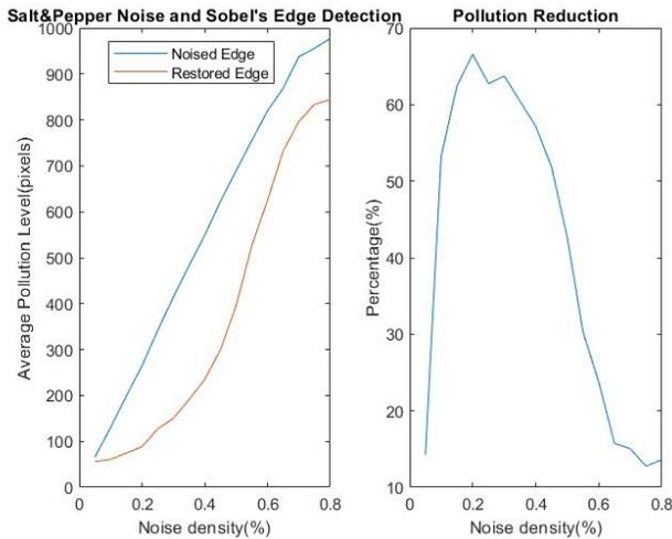
**FIGURE 10:** COMPARISON OF NOISE POLLUTION IN NOISED AND RESTORED EDGES FOR SOBEL EDGE DETECTION ALGORITHM [14]
