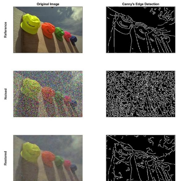
**FIGURE 9** VISUAL COMPARISON OF EDGE DETECTION FOR ORIGINAL, NOISED, AND RESTORED EDGES FOR CANNY EDGE DETECTION ALGORITHM [14]
