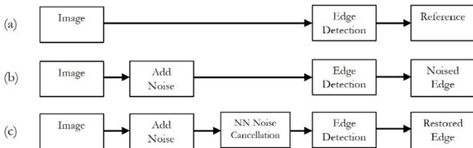
**FIGURE 1: IMAGE PROCESSING DIAGRAM [14]**
