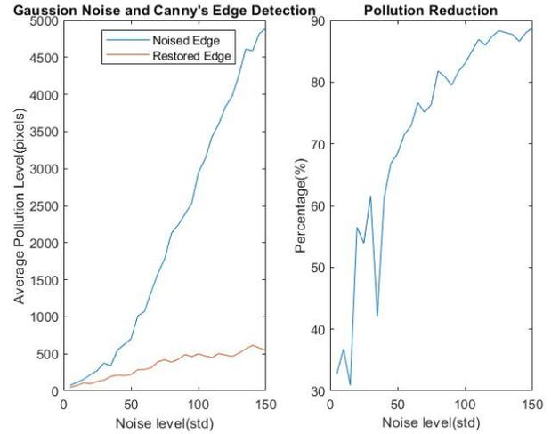
**FIGURE 2: COMPARISON OF NOISE POLLUTION IN NOISED AND RESTORED EDGES FOR CANNY EDGE DETECTION ALGORITHM [14]**
