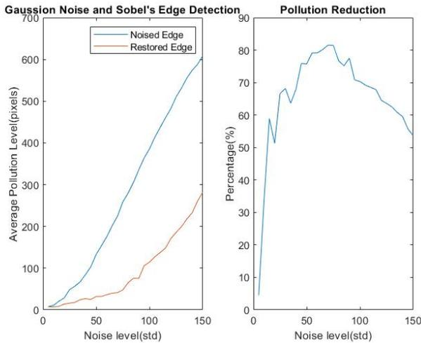
**FIGURE 4:** COMPARISON OF NOISE POLLUTION IN NOISED AND RESTORED EDGES FOR SOBEL EDGE DETECTION ALGORITHM [14]
