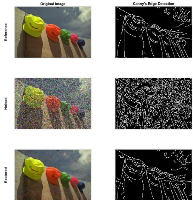
**FIGURE 3: VISUAL COMPARISON OF EDGE DETECTION FOR ORIGINAL, NOISED, AND RESTORED EDGES FOR CANNY EDGE DETECTION ALGORITHM (120 std) [14]**
