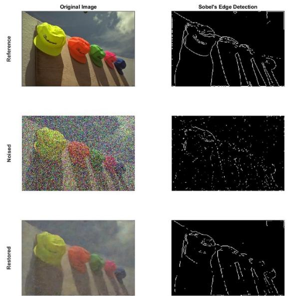
**Figure 11:** VISUAL COMPARISON OF EDGE DETECTION FOR ORIGINAL, NOISED, AND RESTORED EDGES FOR SOBEL EDGE DETECTION ALGORITHM [14]
