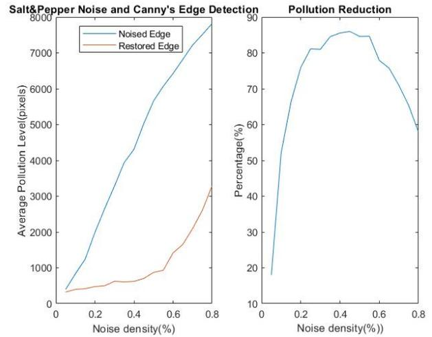
**FIGURE 8:** COMPARISON OF NOISE POLLUTION IN NOISED AND RESTORED EDGES FOR CANNY EDGE DETECTION ALGORITHM [14]
