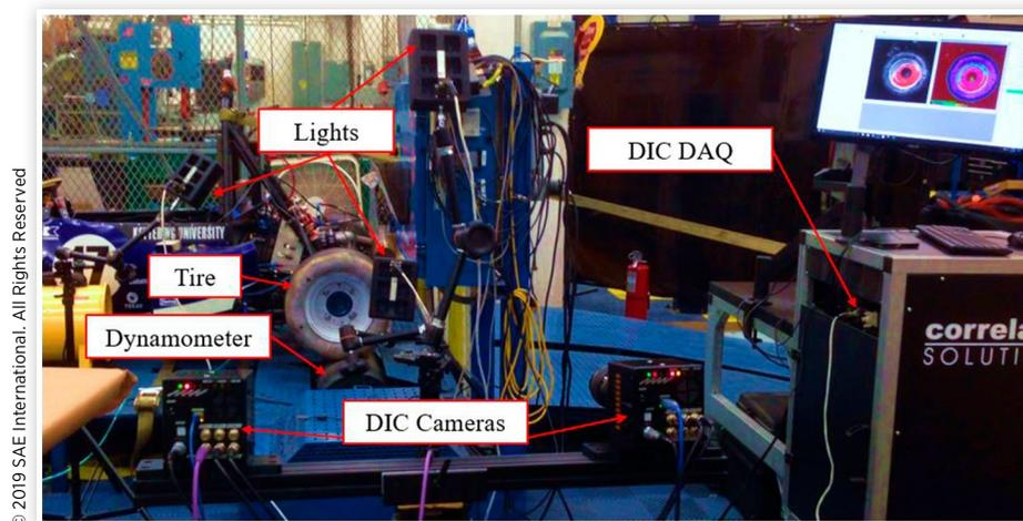
procedure calculates the intrinsic and extrinsic parameters of the high-speed cameras using a triangulation algorithm that compensates for lens distortions. At the end of this calibration procedure, the software defines a three-dimensional coordinate system on the test surface to remove any measurement bias. The experimentation is then performed for non-rotating and rotating conditions of the tire.
