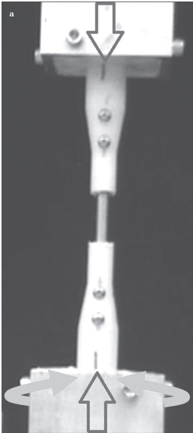
Figure 2: Six fracture analogs were stabilized with 0.5 mm overdrilled collared angle-stable IM nails (Figure 1(c)). The 7.5 mm nails were straight and the endosteal diameter was intentionally oversized by 2.5 mm to ensure the interlocking hardware was challenged as the primary load path. Prior to and after fatigue testing, the constructs were loaded in separate experiments in torsion, compression (a), and four-point bending (b).
