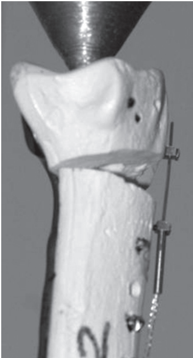
Figure 2: Axial Compression Test. Constructs were axially loaded to a physiologic sub failure load of 250 N using the protocol from [22]. This dorsal view shows the displacement transducer which spanned the fracture gap to record interfragmentary displacement.
