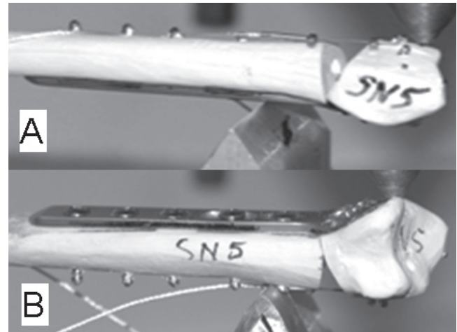
Figure 3: Dorsal and Volar Bending Tests. Three point bending was performed (A) dorsally and (B) volarly to a load of 50 N per [22]. The displacement transducer was again used to record interfragmentary motion.
