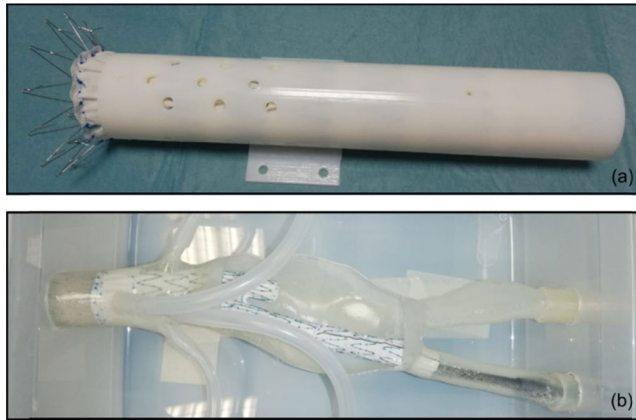
FIGURE 5. In vitro testing setups: Setup A, a non-anthropomorphic phantom (a); and Setup B, a phantom of a short-necked aneurysm (b).
