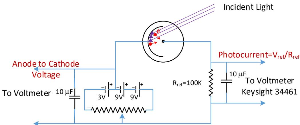
Figure 4. Circuit diagram of the photoelectric effect apparatus
