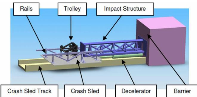
**Figure 4. Impact Attenuator Test Apparatus**
