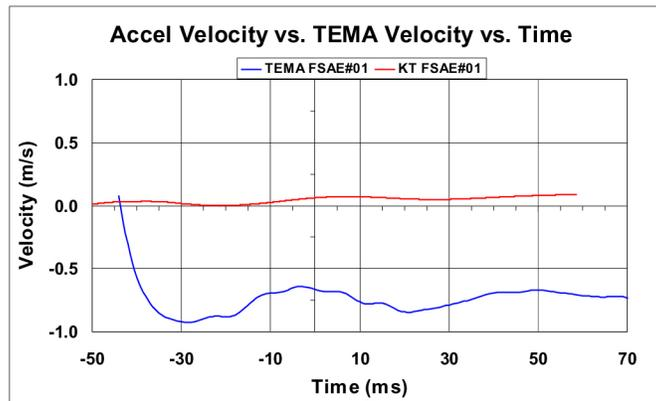
Figure 8. Rebound Portion of Test (TEMA Results Shown In Blue & Accelerometer Integrated Velocity in Red)
