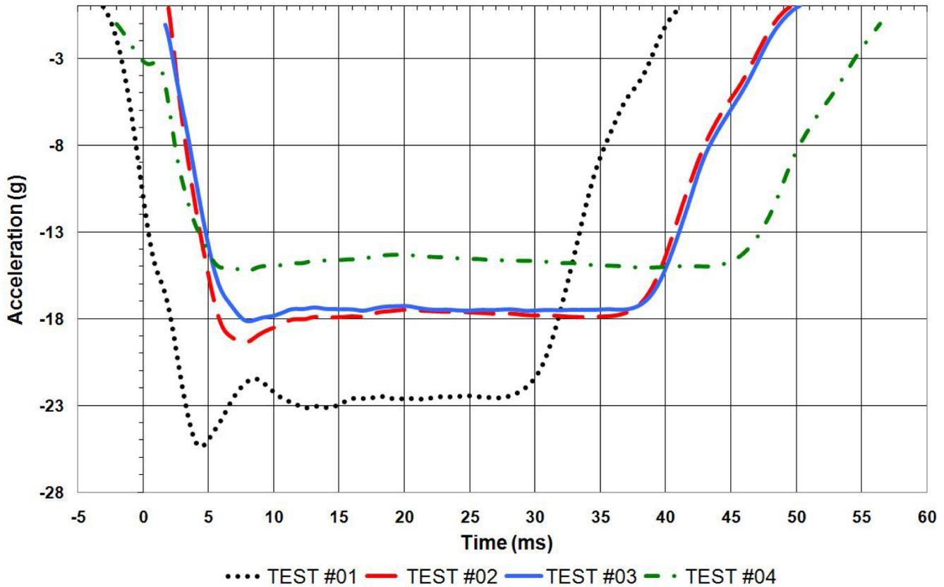
Figure 9. Impact Attenuator Deceleration Results Overlay
