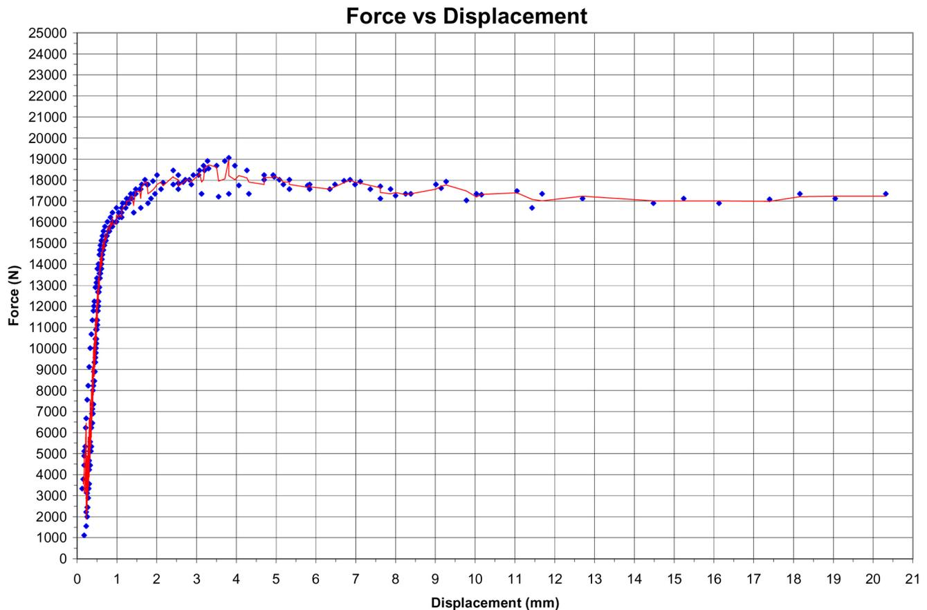
Figure 3. Compression Test Data: Average Load versus Displacement
