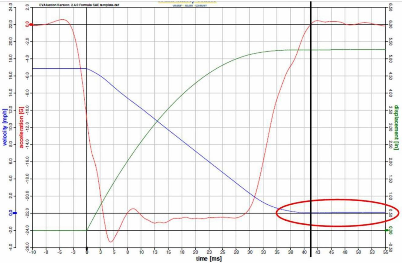
Figure 7. Rebound Phase Accelerometer Error (Circled in Red)
