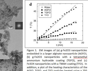
Fe3O4 nanoparticles with a TMAH coating (TFO). In addition, a plot of the heating characteristics of the AGFO, TGFO, and TFO particles heated using a 250 Oe ac magnetic field driven at 125 kHz. The heating curve for de-ionized water is also provided as a reference. The solid lines drawn through the data are intended as guides to the eye. Figures taken from Vaishnava *et al*, J. Appl. Phys. **102**, 063914.
