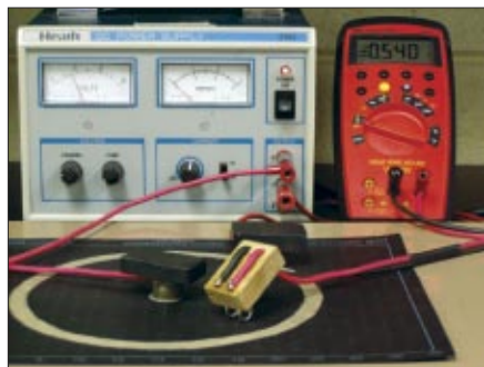
Fig. 2. The experimental apparatus features the electric field probe: a small block of wood with two electrodes made from upholstery pins. For scale, the grid spacing on the conducting paper is 1 cm. The power supply (Heath 2732) and multimeter (Metorman 38XR) are standard lab equipment.
