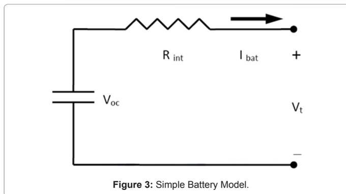
Figure 3: Simple Battery Model.
