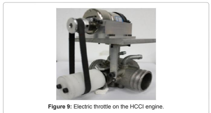
Figure 9: Electric throttle on the HCCI engine.
