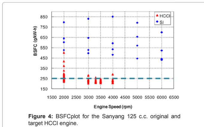
Figure 4: BSFC plot for the Sanyang 125 c.c. original and target HCCI engine.
