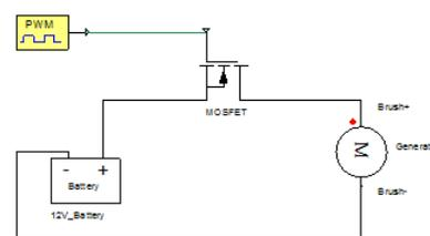
Figure 13: Magnetizing current control circuit.
