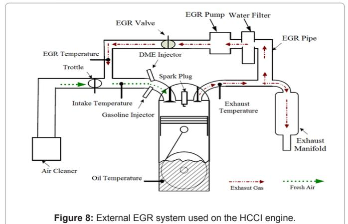
Figure 8: External EGR system used on the HCCI engine.
