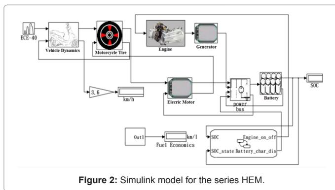
Figure 2: Simulink model for the series HEM.
