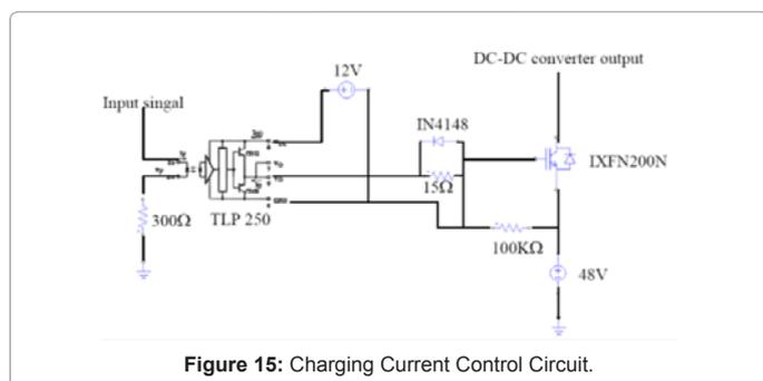
Figure 15: Charging Current Control Circuit.
