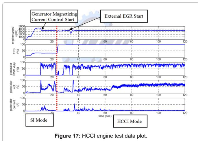
Figure 17: HCCI engine test data plot.
