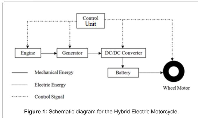
Figure 1: Schematic diagram for the Hybrid Electric Motorcycle.
