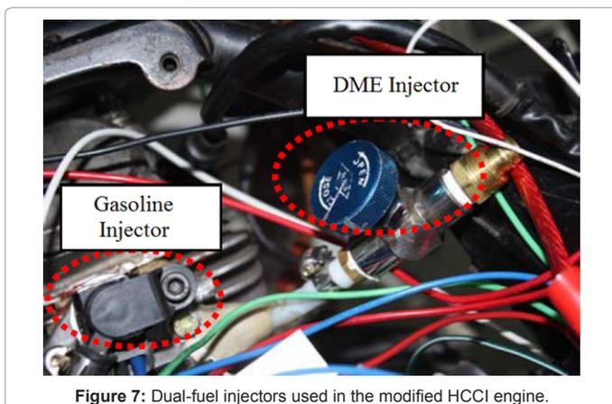
Figure 7: Dual-fuel injectors used in the modified HCCI engine.
