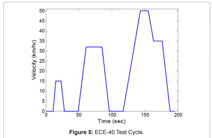
Figure 5: ECE-40 Test Cycle.
