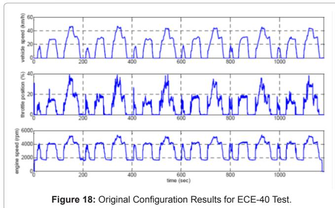
Figure 18: Original Configuration Results for ECE-40 Test.
