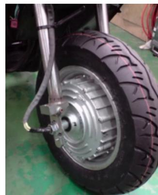
Figure 16: Hub Motor as Front Wheel Drive Unit.
